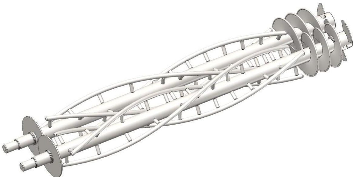
Figure 2. Overview of the computer model of the kneading body of a continuous kneading machine Source: compiled by the author.
